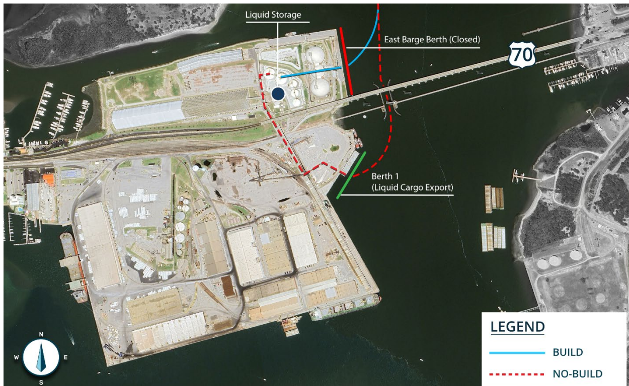
Figure 2. With the East Barge Berths closed, liquid barges must navigate to Berth 1 beneath the Newport River Bridge, which requires a skilled pilot and fair weather. Liquid cargo must travel a longer distance to be unloaded, use inefficient temporary equipment at Berth 1, and there is no capacity to stage more than one barge for unloading at a time nor load an export ship while barges are unloading.
