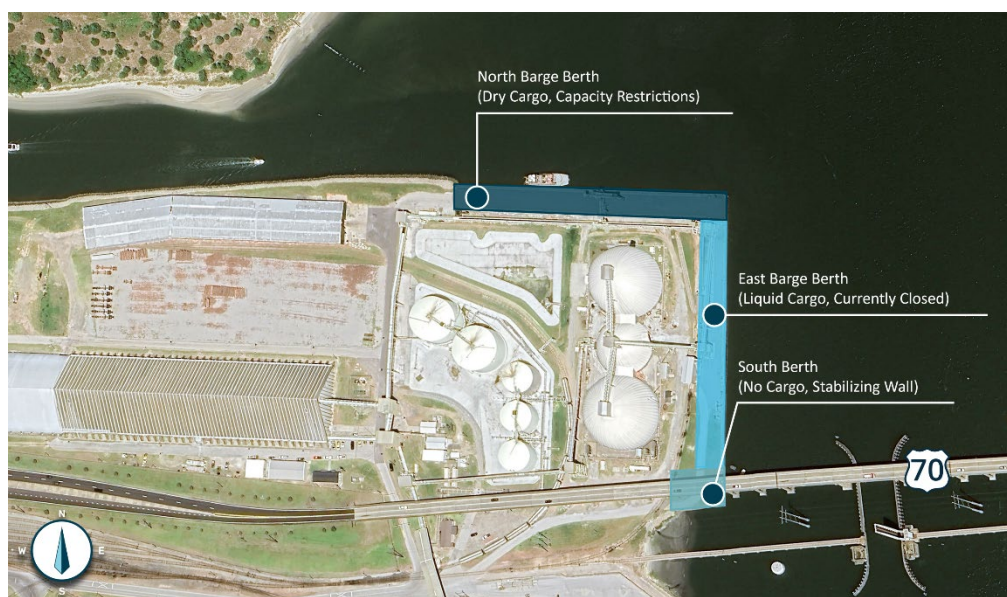
Figure 1. The project scope includes reconstruction of the Phosphoric Acid Terminal North, East, and South Berths to restore state of good repair, safe working conditions, and full berthing capacity.
